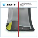
Normal inflation conditions at 200kPa. The yellow area indicates reinforced, thicker sidewall.
