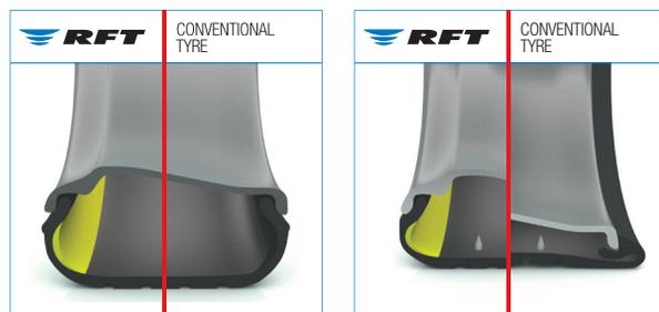
Normal inflation conditions at 200kPa. The yellow area indicates reinforced, thicker sidewall.
