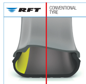
Normal inflation conditions at 200kPa. The yellow area indicates the reinforced, thicker sidewall.
